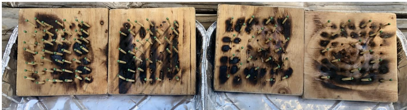
Figure 1. A series of pegboards, left to right, with 49, 32, 35 and 16 matches evenly distributed across the board. It is recommended to burn these left to right, starting with the board that has the fewest matches.
